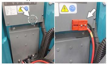
7. Re-install batteries and connect kit battery cable harness to batteries as shown.
