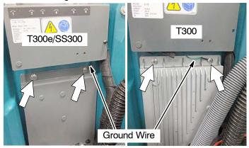
6. Connect battery cable connector to panel using two screws supplied with kit as shown.
