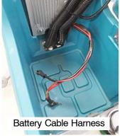
Remove the top two screws from the electrical panel and carefully lower panel.
