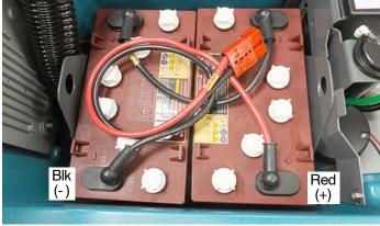
8. Connect battery cable connectors together.
