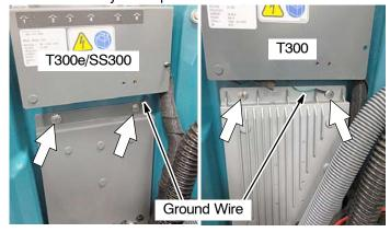
3. Disconnect battery cable harness from electrical panel and discard cable harness. Save terminal boots.
